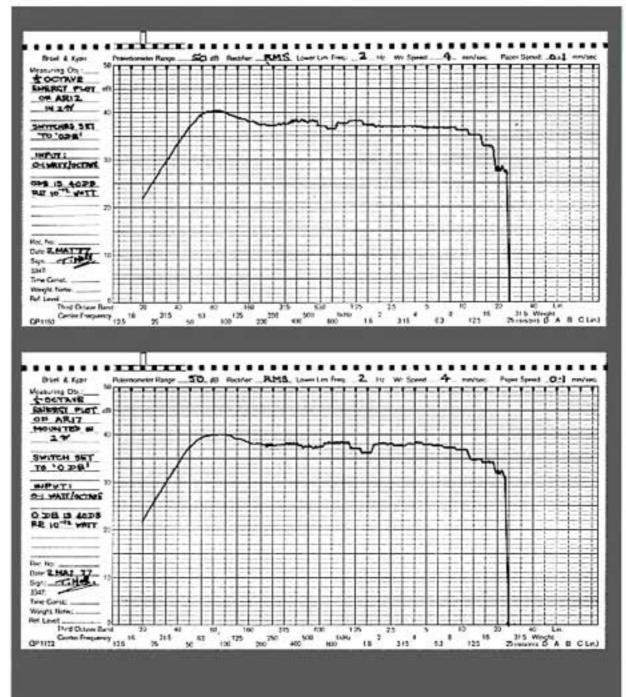
1/3 octave energy plots for the AR 12 (above) and the AR 17 (below) illustrate the AR design philosophy. While the AR 12 is capable of handling more power, note that the energy response for both speakers is virtually the same from 20Hz to over 20kHz. The "flat" curve indicates a high degree of accuracy. or "truth in listening."
