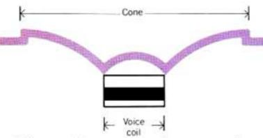
The speaker cone can be mounted loosely and is therefore extremely responsive. Bass harmonic distortion is greatly reduced. Low frequency response is uniform and extended. Far better bass response can be extracted from a small enclosure and thus the entire speaker system gives extremely truthful reproduction.
